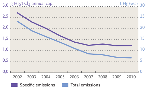
WCC - Chlor-Alkali Industry / Total mercury emissions (air + water + products) (for USA/Canada/Mexico, Europe, India and Brazil/Argentina plus 1 Uruguayan and 3 Russian plants from 2005 onwards)
