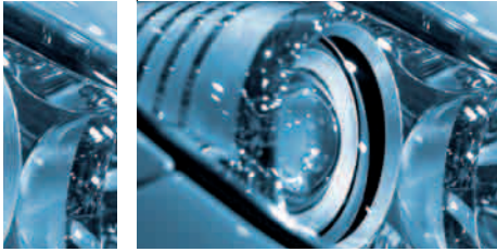
Modern car headlights can be beautifully styled thanks to the plastic polycarbonate
